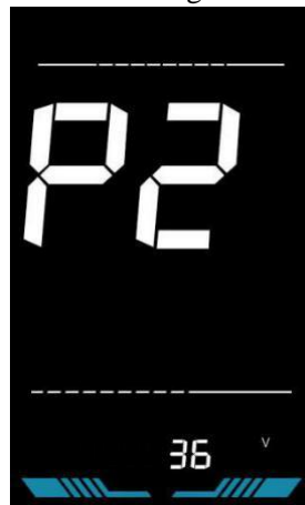
Figure 6-2 Rated voltage setting interface
