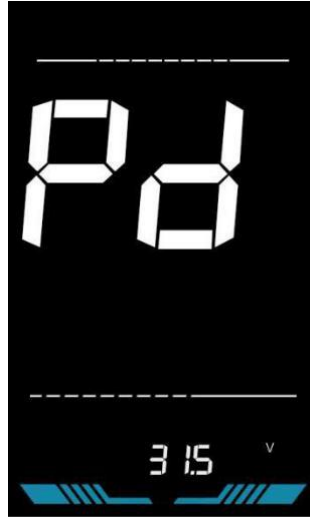
Figure 6-13 Battery under voltage value setting interface
